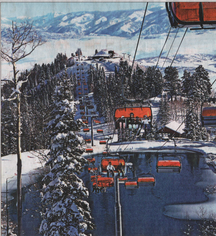
The Orange Bubble Express lift chairs at Canyons Village at Park City feature heated seats and a bubblelike enclosure. VAIL RESORTS
